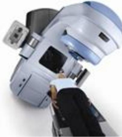
A **Linear Accelerator** (also called a **LINAC**) is an electrical device used to produce high energy X-rays which are then manipulated to deliver external beam radiation treatments for patients with cancer. The produced x-ray beam comes out of the part of the accelerator called the gantry. This gantry rotates around the patient while delivering the radiation treatment.
